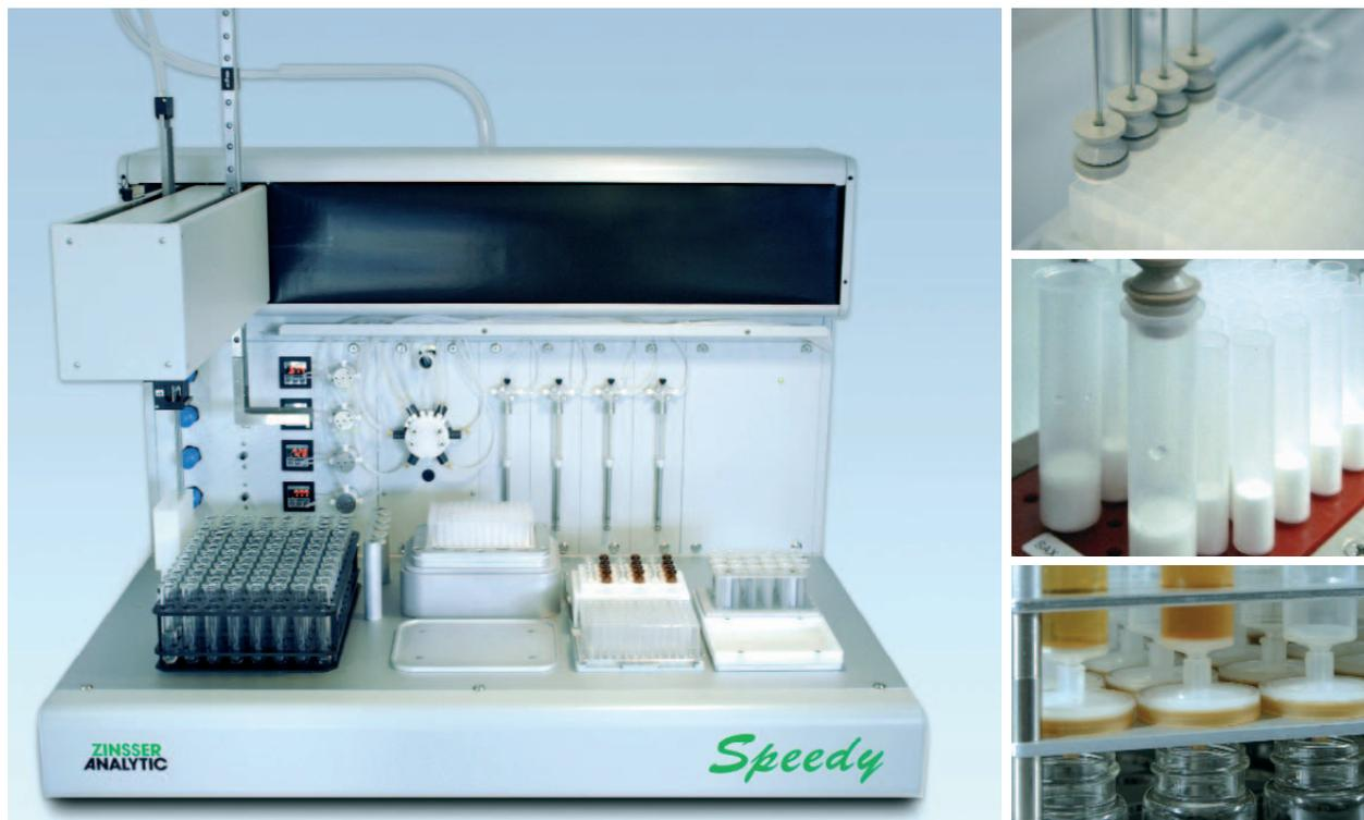
SPEEDY® is an automatic system for solid phase extraction and filtration, which can handle filtration plates and SPE plates or cartridges.
