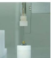
Zinsser Analytic has developed ProCrys Meso Plus, a new liquid handling platform for the preparation of 96 in-meso (or cubic phase) proteins, for reliable and easy preparation of protein plates. The new ProCrys Meso superceeds any other system on the market. With high precision – better than  $20\mu m$  – the system places the extremely viscous lipid cubic phase (LCP) proteins on the crystallization plates controlled by sophisticated mechanical and optical sensors.
